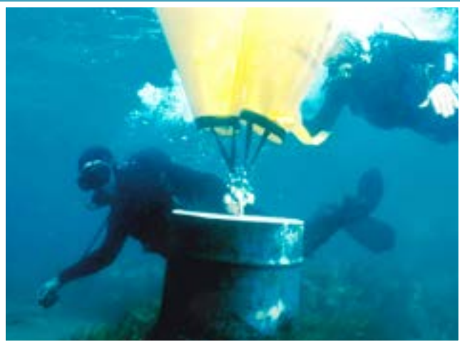
200kg drums were moved by club members using airbags
